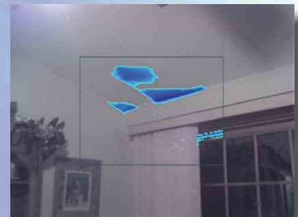
IR/visible alarm For displaying only temperatures that fall above, below, or in between a specified range as IR image, leaving the rest of the scene as a fully visible light image.
