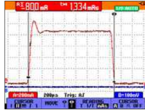
Current-over-time measurement using cursors, in dual channel mode on the Fluke 199CM
