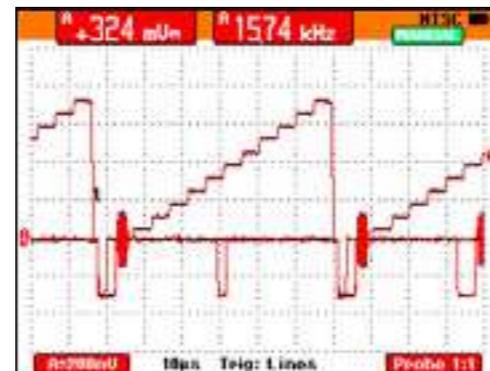
Smart averaging shows the averaged curve of repeated signal parts, as well as incidental deviations
