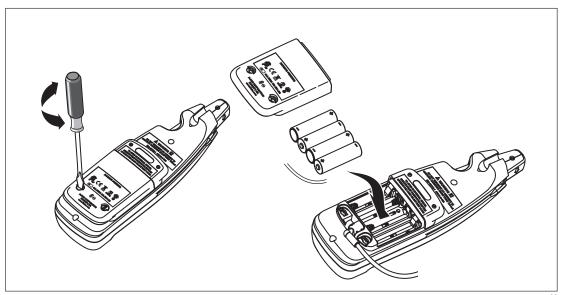
Figure 2. Battery Replacement
