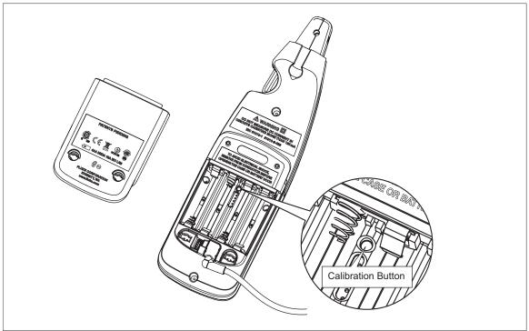
Figure 4. Accessing the Calibration Button
