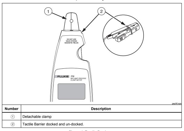
Figure 1. Tactile Barrier
