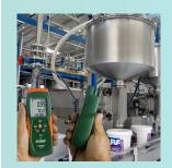
Measures Formaldehyde concentration, Air Temperature, and Humidity. Adjustable audible alarm feature is excellent for checking indoor air quality in buildings.
