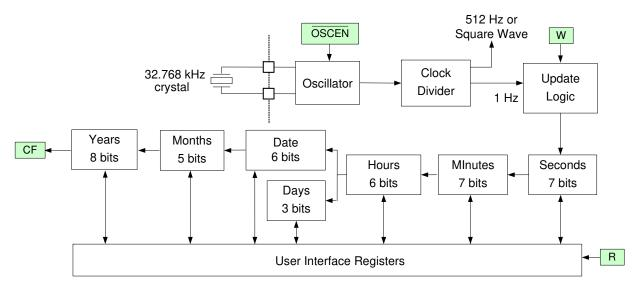
Figure 7. Real-time Clock Core Block Diagram
