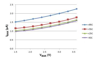
The minimum  $V_{BAK}$  voltage varies linearly with temperature. The user can expect the minimum  $V_{BAK}$  voltage to be 1.23 V at +85 °C and 1.90 V at -40 °C. The tested limit is 1.55 V at +25 °C.
