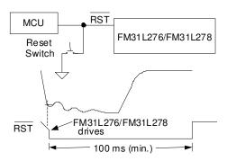
**Note** The internal weak pull-up eliminates the need for additional external components.
