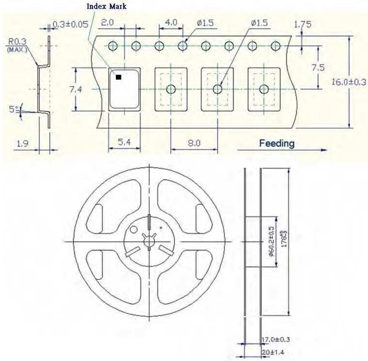
1. 230mm minimum leafer which consist of carrier and/or tape followed by a minimum of 160mm of empty carrier tape sealed with cover tape.
