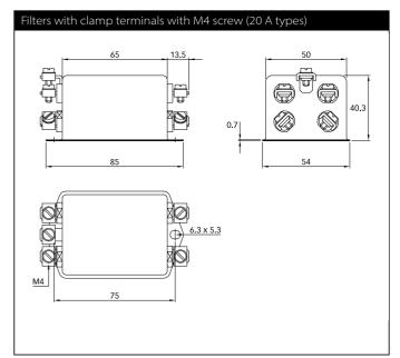
All dimensions in mm; 1 inch = 25.4 mm Tolerances according: ISO 2768-m / EN 22768-m
