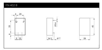
All dimensions in mm; 1 inch = 25.4 mm Tolerances according: ISO 2768-m/EN 22768-m
