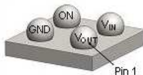
Figure 4. 1 x 1mm WLCSP Bumps Facing Up
