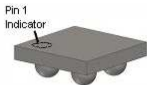
Figure 3. 1 x 1mm WLCSP Bumps Facing Down
