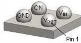
Figure 4. 1 x 1mm WLCSP Bumps Facing Up
