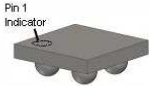
Figure 3. 1 x 1mm WLCSP Bumps Facing Down
