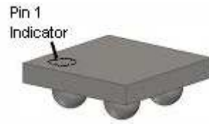
Figure 4. WLCSP Bumps Facing Down (Bottom View)
