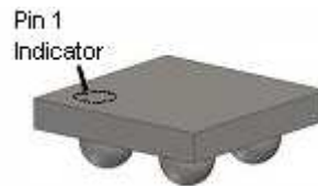
Figure 4. WLCSP Bumps Facing Down (Bottom View)
