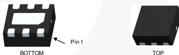
Figure 1. 2 mm x 2 mm Molded Leadless Package (MLP)
