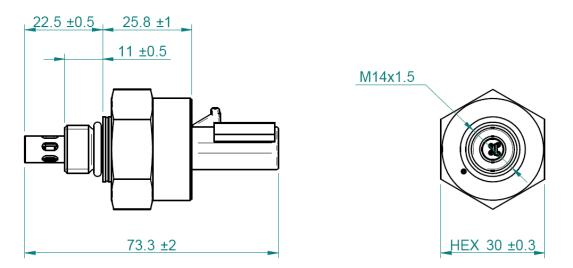
All dimensions are millimeters (mm). Mating connector type is FCI female receptacle ref. 54200409 (black-sealed). Sensor body is stainless steel.
