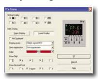
Control FPWIN Pro offers easy-to-use dialogs to comfortably configure the PLC, e.g. the screen display of the FP-e.
