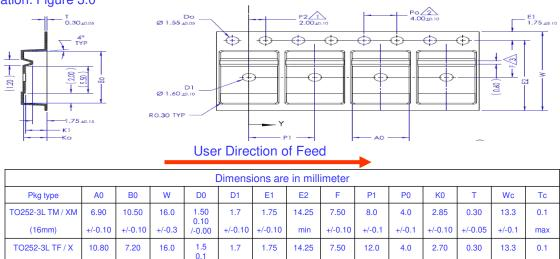
+/-0.10 Notes: A0, B0, and K0 dimensions are determined with respect to the EIA/Jedec RS-481 rotational and lateral movement requirements (see sketches A, B, and C).
