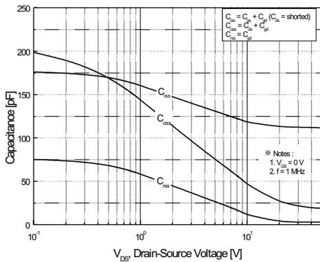
Figure 5. Capacitance Characteristics
