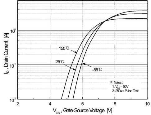
Figure 2. Transfer Characteristics
