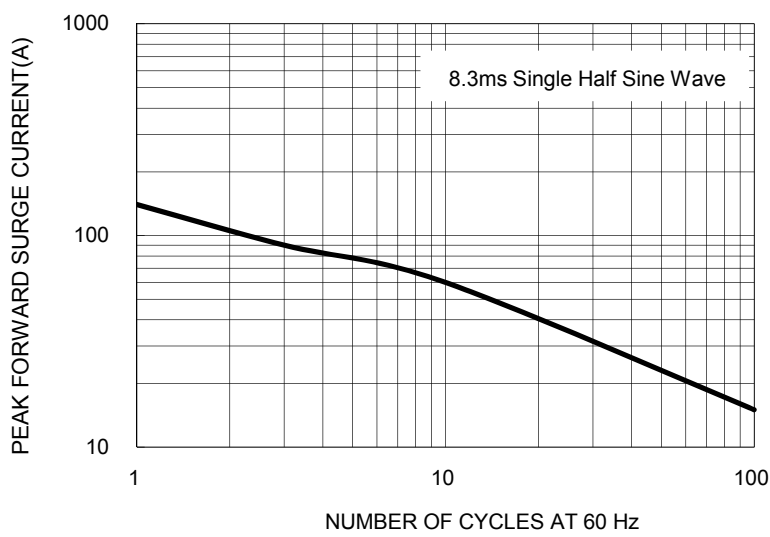
FIG. 3 MAXIMUM NON-REPETITIVE PEAK FORWARD SURGE CURRENT
