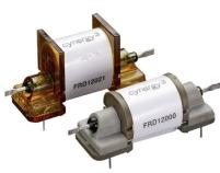
An open frame RF reed relay with 8kV isolation and 6A (at 30MHz) carry current, the FRD12000 series has been used many HF radio system specifications over the years, with applications in commercial maritime (GMDSS) equipment and military HF radio units worldwide. The use of vacuum reed switches with rhodium contacts offers high isolation voltages, low contact resistance and long operating lifetime.
