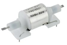
A complete RF screen around the coil assembly for a low loss transmission path, results in better carry current at elevated temperatures for this open frame series. An anti-corona sleeve is tted around the reed switch for improved RF voltage isolation. This type is widely used in HF Antenna Tuning Unit (ATU) applications.
