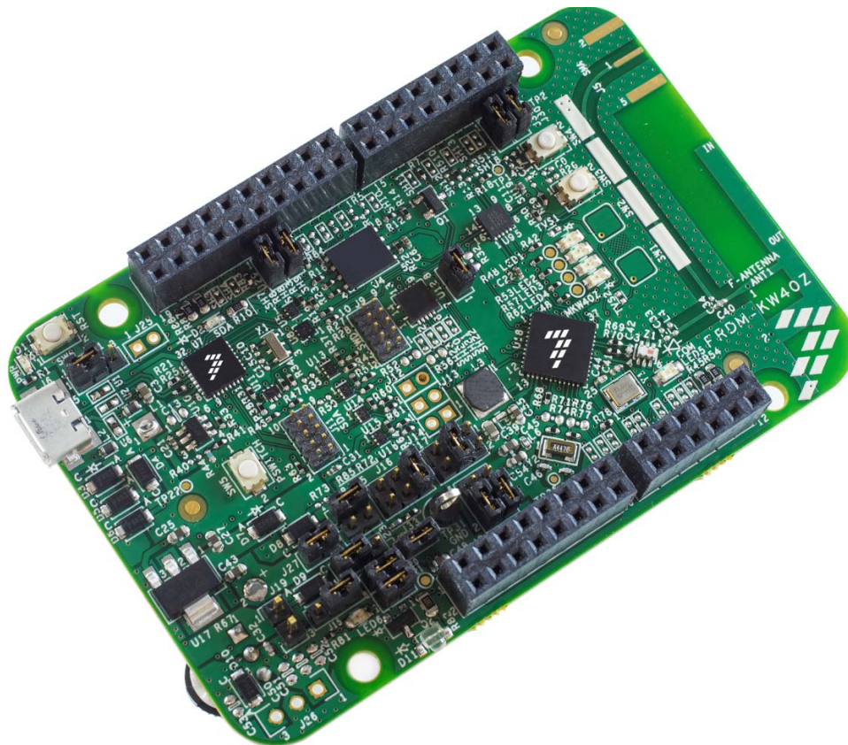
Figure 1. FRDM-KW40Z Freedom development board
