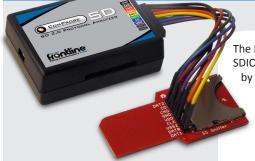
The Frontline SD Protocol Analyzer includes powerful Frontline software and the SD/SDIO/SPI/ MMC hardware interface.
