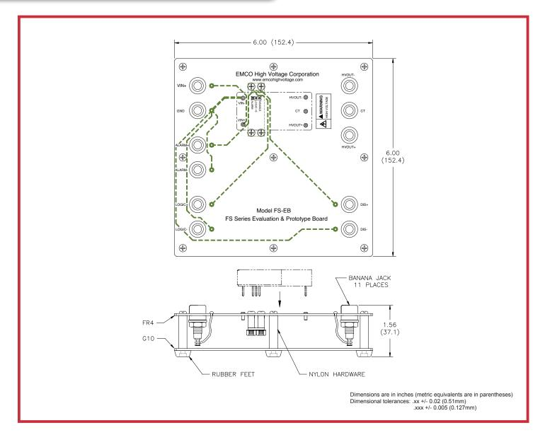
This FS-EB evaluation board provides a convenient package to use any FS Series high voltage power supply without having to fit it onto a PC board. The board provides for easy prototyping and evaluation.
