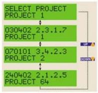
In 'Standalone Mode', the FS2009 is controlled via the push buttons on the front panel of the programmer - no PC connection is required. The programmer LCD and the LED Status Indicators are used to display the current status of the programmer. It is possible to select from 1 of 64 previously uploaded Programming Projects and then to repeatedly execute this project to program a batch of devices.
