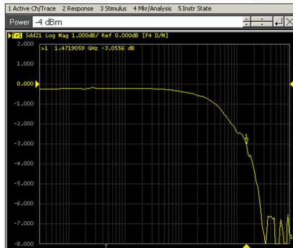
Figure 18. USB Path SDD21 Insertion Loss Curve
