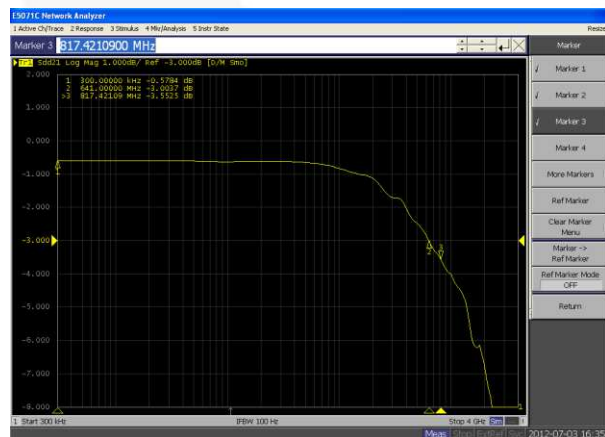
Figure 18. USB Path SDD21 Insertion Loss Curve
