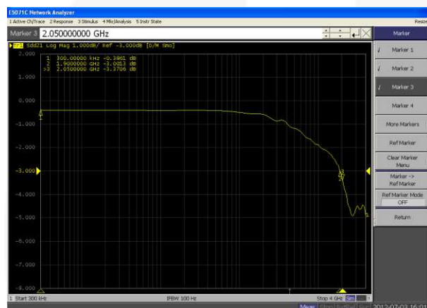
Figure 17. MHL Path SDD21 Insertion Loss Curve
