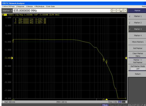
Figure 18. USB Path SDD21 Insertion Loss Curve
