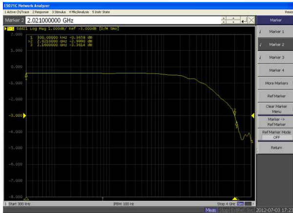
Figure 17. MHL Path SDD21 Insertion Loss Curve
