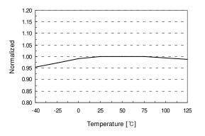
Figure 4. Operating Frequency (fosc) vs. T<sub>A</sub>
