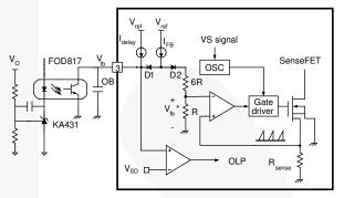
Figure 14. Valley Switching Pulse-Width Modulation (VS-PWM) Circuit
