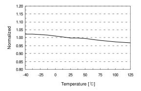
Figure 8. Shutdown Feedback Voltage (V<sub>SD</sub>) vs. T<sub>A</sub>
