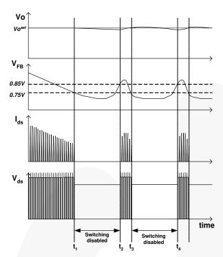
Figure 18. Burst-Mode Operation
