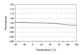
Figure 5. Peak Current Limit (I<sub>LIM</sub>) vs. T<sub>A</sub>
