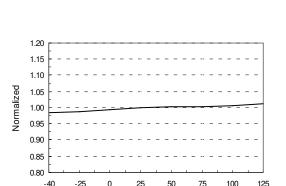
Figure 6. Start Threshold Voltage (V<sub>START</sub>) vs. T<sub>A</sub>
