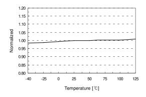
Figure 7. Stop Threshold Voltage (V<sub>STOP</sub>) vs. T<sub>A</sub>
