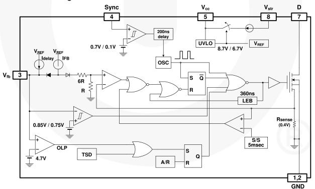
Figure 2. Internal Block Diagram
