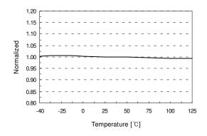
Figure 9. Maximum Duty Cycle (D<sub>MAX</sub>) vs. T<sub>A</sub>
