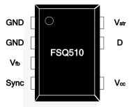
Figure 3. Pin Assignments
