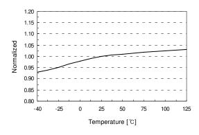
Figure 11. Shutdown Delay Current (IDELAY) vs. TA
