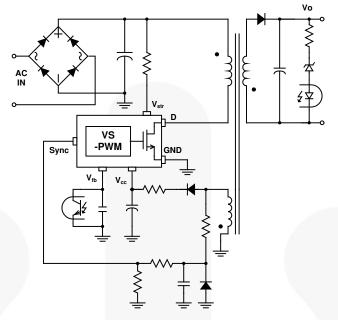
Figure 1. Typical Application Circuit
