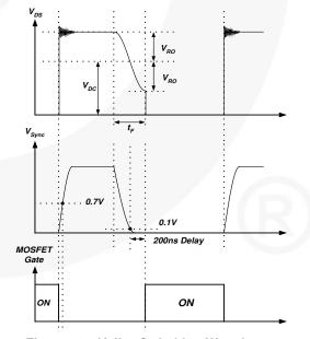
Figure 15. Valley Switching Waveforms
