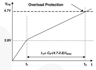
Figure 17. Overload Protection
