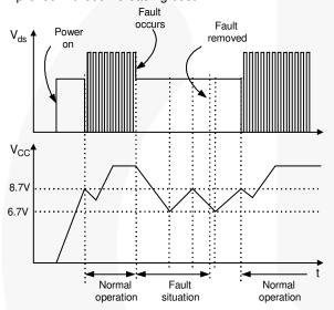
Figure 16. Auto Restart Protection Waveforms
