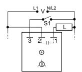
V = Voltage S1 = Optional low current switch L = Load
