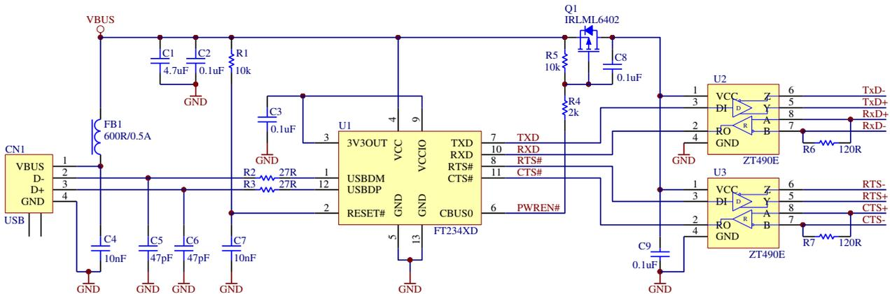
**Figure 7.3 USB to RS422 Converter Configuration**
