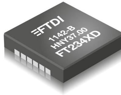
The FT234XD is a USB to serial UART interface with optimised packaging (3mm x 3mm 12 pin DFN) for smaller PCB designs and the following advanced features:
