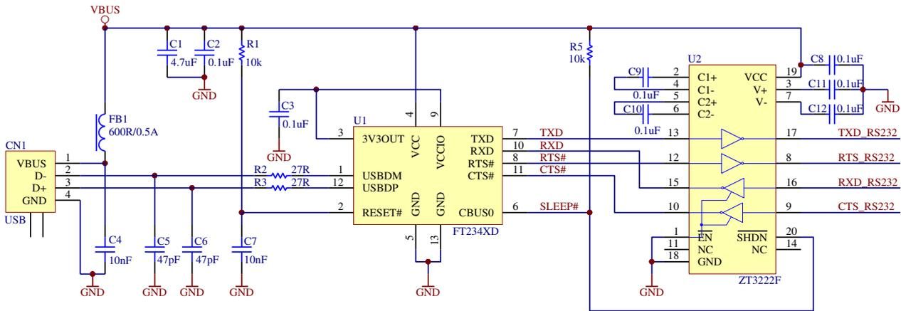
**Figure 7.1 Application Example showing USB to RS232 Converter**
