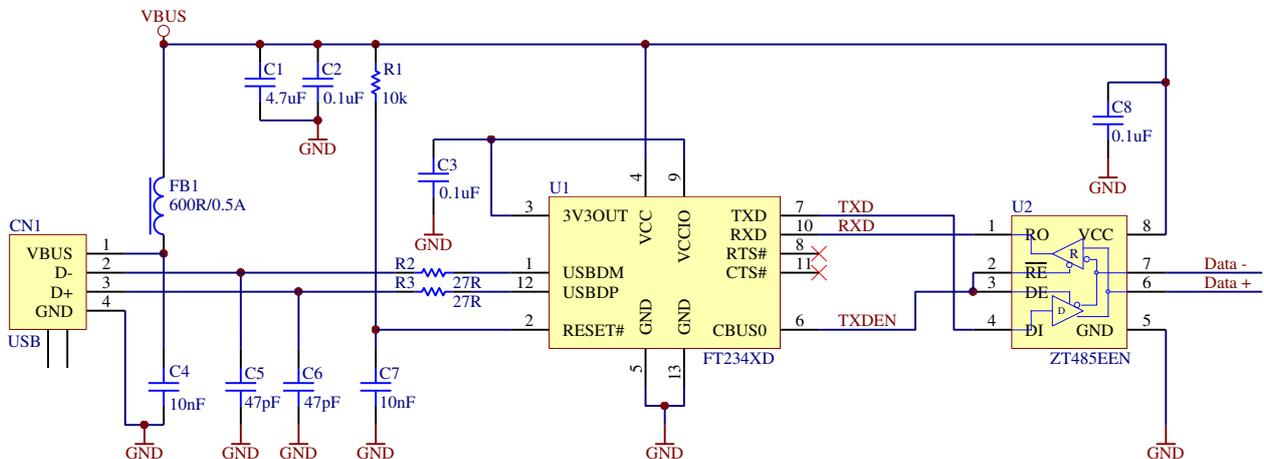
**Figure 7.2 Application Example Showing USB to RS485 Converter**
