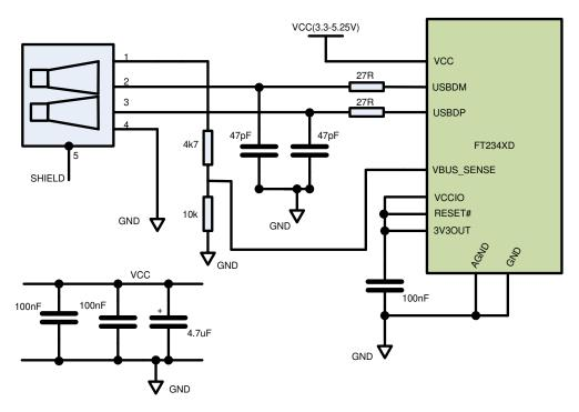
Figure 6.2 Self Powered Configuration
