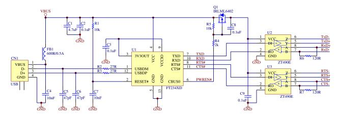
Figure 7.3 USB to RS422 Converter Configuration
