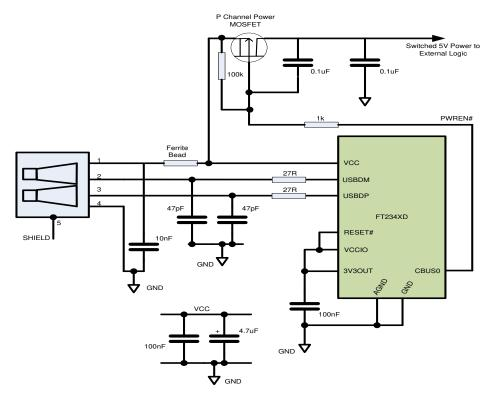
Figure 6.3 Bus Powered with Power Switching Configuration
