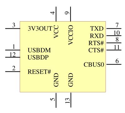
Figure 3.1 DFN Schematic Symbol
