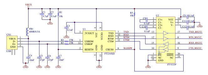
Figure 7.1 Application Example showing USB to RS232 Converter
