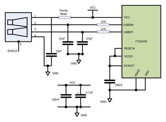
Figure 6.1 Bus Powered Configuration
