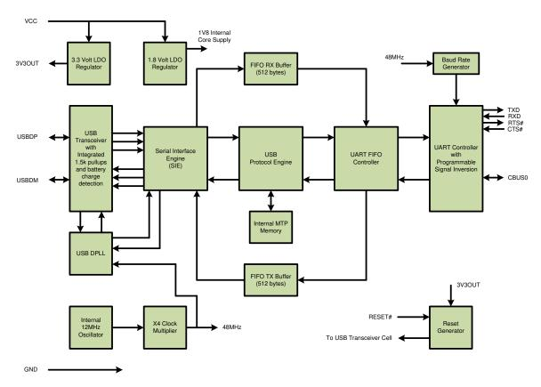
Figure 2.1 FT234XD Block Diagram
