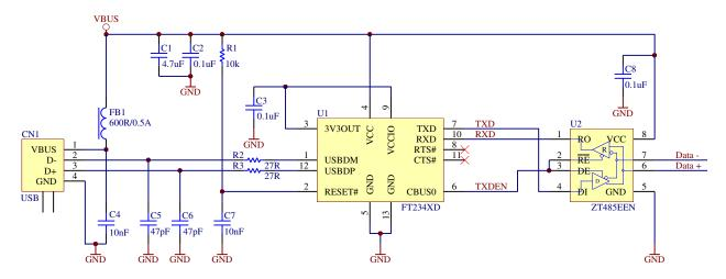
Figure 7.2 Application Example Showing USB to RS485 Converter
