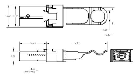
Figure 5 – FTLD10C mechanical drawing
