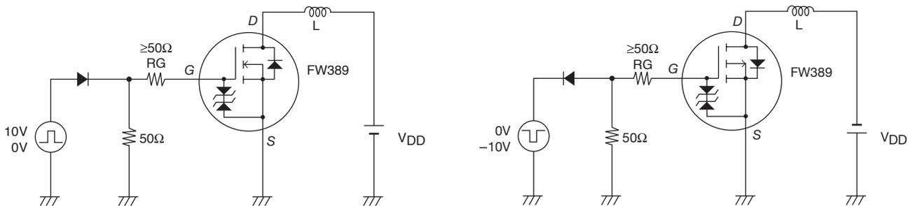
Fig.2 Switching Time Test Circuit
