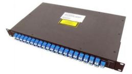
Forty channels DWDM module is a passive optical add/drop multiplexer/demultiplexer designed for metro access applications that represent the state of the art in fiber optics design. Finisar's forty channels DWDM design maps the two added/dropped channel of forty wavelengths with 100GHz channel spacing into two-fiber paths, going in opposite directions into the network.
