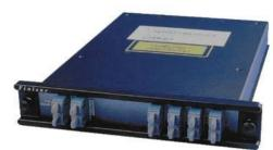
CWDM MUX/DEMUX-4-EX plug-in module is a passive optical multiplexer /demultiplexer designed to add CWDM wavelength channels to an existing backbone ring. The MUX/DEMUX multiplexes and demultiplexes four CWDM wavelengths from a two-fiber ring, going in opposite directions into a network. The module also includes an expansion port that allows adding more CWDM channels for future upgrade.
