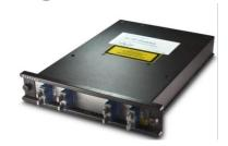
OADM-1 plug-in module is a passive optical multiplexer /demultiplexer designed to add and drop CWDM channels into an existing backbone ring. The module multiplexes and demultiplexes one CWDM wavelength from a two-fiber ring, going in opposite directions into a network (east/west).
