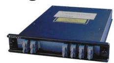
OADM-4 plug-in module is a passive optical multiplexer /demultiplexer designed to add and drop CWDM channels to an existing backbone ring. The module multiplexes and demultiplexes four CWDM wavelengths from a two-fiber ring, going in opposite directions into a network (east/west).
