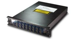
Sixteen channel FWSFDMUXDwxxyy DWDM Plug-in module is a passive optical multiplexer designed for metro access applications that represent the state of the art in fiber optics design. This MUX module multiplexes sixteen DWDM wavelengths of 100GHz channel spacing into a ring or point-to-point network.
