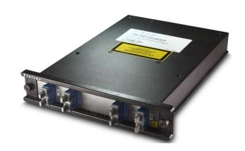
One channel FWSFOADMD1xxyy DWDM plug-in module is a passive optical add/drop multiplexer designed for metro access applications that represent the state of the art in fiber optics design. Finisar's unique one channel DWDM design maps one pair of add/drop channels of same wavelength with 100GHz channel spacing into two-fiber paths, going in opposite directions into a network (east/west).
