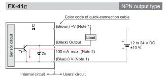
Notes: 1) The quick-connection sub cable does not have +V (brown) and 0 V (blue). The power is supplied from the connector of the main cable.
