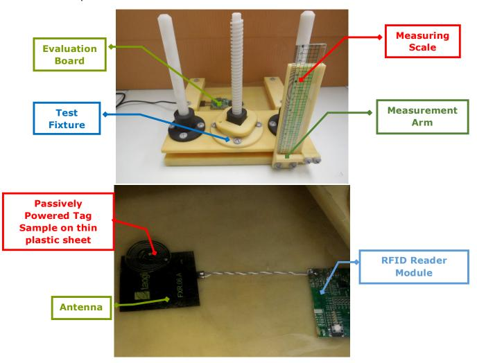
The test sample is placed on a thin sheet of plastic connected to the movable part of the fixture. Then the distance is carefully adjusted until the reader can no longer read the sample, thus the maximum interrogation distance is displayed in the ruler.
