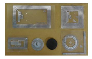
The Tag-it HF-I Plus Transponder Inlay family of Texas Instruments RFID is based on the ISO/IEC 15693 standard for contactless integrated circuit cards (vicinity cards) and ISO/IEC 18000-3 standard for item management.
