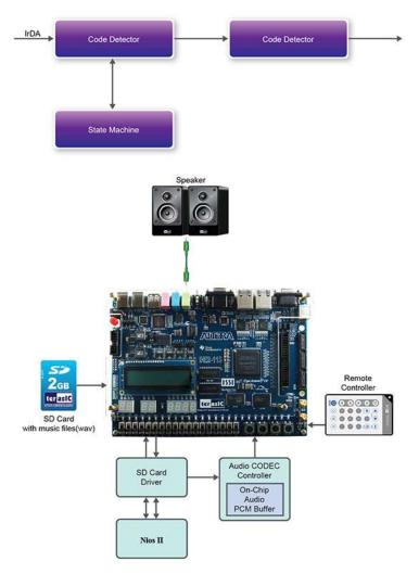
• Support working with DE2-115 / DE1-SoC development kits which includes the IR receiver.
