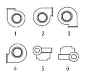
Mounting positions 1 - 4 are possible. If the motor is installed on anti-vibration mounts, the motor weight is given additional support by an elastic element. Details of the mounting position must therefore be provided.
