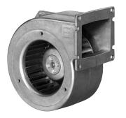
AC single inlet, forward curved centrifugal blower. Via a bracket, the integrated external-rotor motor is mounted on one side of the housing.
