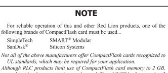
cards with a larger capacity can be used. They MUST be formatted to 2 GB and use the FAT 16 file system. It is recommended to format the CF card using the format utility from within Crimson.
