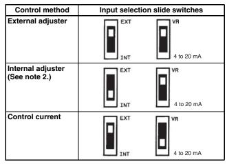
Note: 1. The input selection slide switches are factory-set to internal adjuster input. Change the setting of the switches for the input method required.
