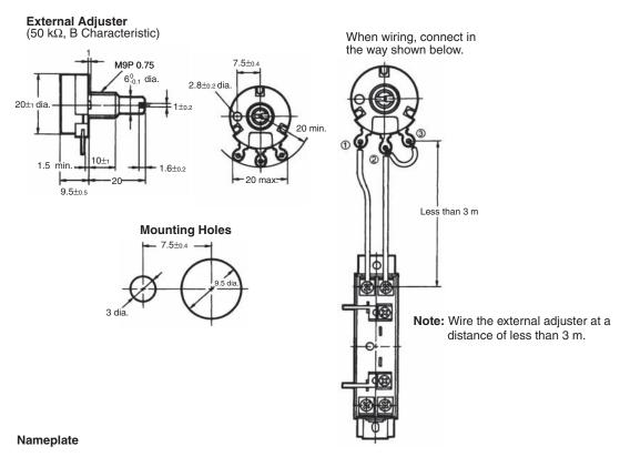
Note: When using the external adjuster for input, be sure to set the input selection slide switches accordingly.
