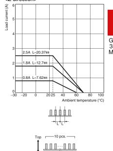
• Thirty Relays are soldered to the PCB at each given spacing.
