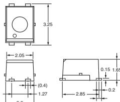
Unless otherwise specified, the dimensional tolerance is  $\pm 0.2$  mm.**Actual Mounting Pad Dimensions**
