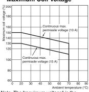
Note. The "maximum voltage" is the maximum voltage that can be applied to the relay coil.
